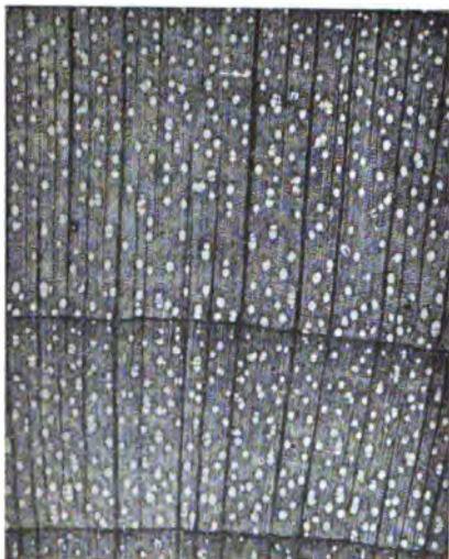
FIG. 1. — Cross-section of Diffuse-Porous Wood. (Hard Maple.) (Bull. 126, U. S. For. Ser.)
